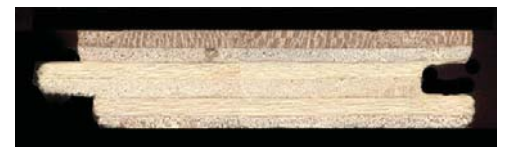
Cross section of engineered wood flooring.
